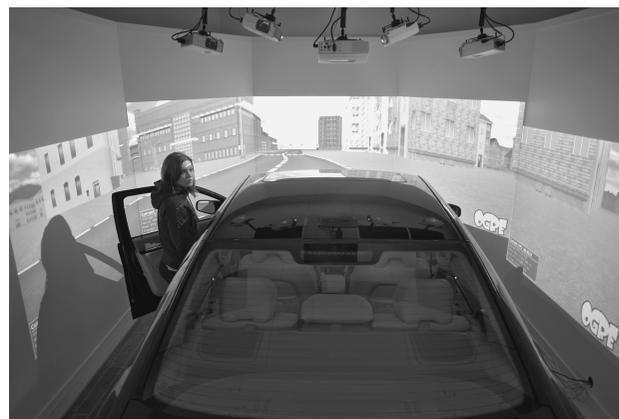
Figure 1. A game based driving simulator. Photo: University of Skövde.
